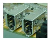
The **three IEEE 1394a ports** on both the IT7 and the AT7 incorporate many features, including support up to 63 peer-to-peer devices, operating speeds of 100 Mbps to 400 Mbps depending on cable type, connects over short and long distances, and supports both
